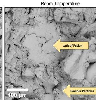
The fracture surfaces consistently show evidence of brittle fracture, such as planar surfaces. The brittle fracture surfaces examined feature perpendicular cracks, which may be due to the hatching pattern used during printing. The presence of larger smooth surfaces and unmelted powder particles on the fracture surface indicate a lack of fusion in the build, which contribute to the lower than expected mechanical properties.
