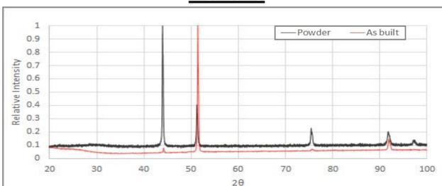
Analyses show higher relative peak intensity of the as-built sample in the (200) plane, indicating a strong crystallographic texture in the observed columnar grains.
