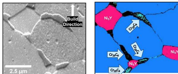
EDS and EBSD indicate the presence of M<sub>23</sub>C<sub>6</sub> carbides, a Ni<sub>5</sub>Y phase, and a Ni-Cr matrix. Y and O were detected but not present in fine Y<sub>2</sub>O<sub>3</sub> dispersoids. The presence of Si and decreased amount of Ti and Al indicate inadequate processing.
