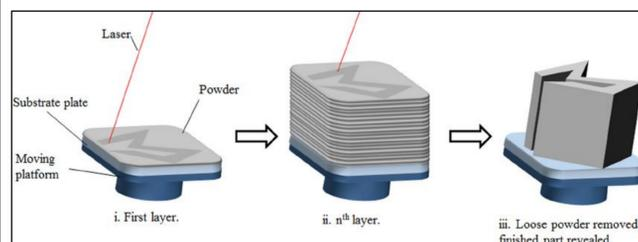
DMLM parts solidify directionally due to thermal gradients. Annealing can relieve resultant residual stresses.
