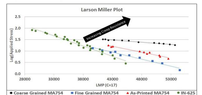
Comparison to literature suggests initial creep testing occurred in low creep exponent region where fracture by cavitation would be expected.
